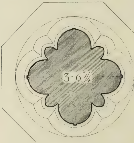
FIG. 1039.—St. John the Baptist's, Perth. Section of Pier of Choir.
